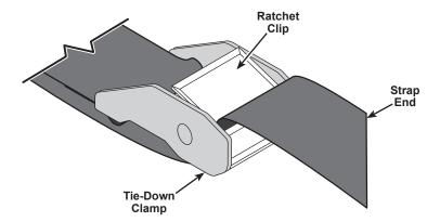
8. To release the strap, push on the ratchet clip and pull the strap loose.
